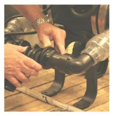
Step 2. Remove the suction flange tee and washers by removing the 2" flange v-clamps. You may have to spread the tee and elbow flanges on one side of the tee and then the other while working the flange tee and washers free.
