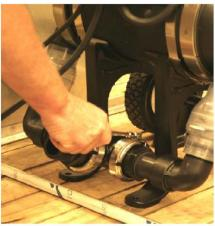
Step 6. Install the flange tee and sealing washers, then install and tighten the flange tee v-clamps. If required follow the same procedures to change the discharge check valves. When completed loosen the pump base v-clamps and rotate the suction and discharge and base assemblies to their original position and make sure all v-clamps are tight.
