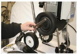
Step 4. Use a 1/2" drive or a crescentwrench to unscrew the diaphragm retaining nut, lower standard and diaphragm from the piston.
