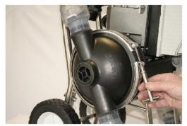
Step 2. Remove the Pump Base V Clamp by unscrewing the Tee Handle all the way
