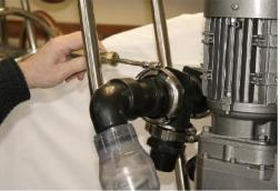
Step 5. Use a little teflon grease to hold the gaskets in place while you align the Pump Base & Valves Assembly. Hold the Pump Base tight to the diaphragm with your body while you fit and tighten the large pump base V Clamp. Make sure the Pump base, the diaphragm and the pump frame are aligned before tightening the V Clamp. Re-install the 2" Flange V Clamps on the suction and discharge Tee before starting to change the other diaphragm.
