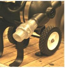
Step 4. Screw the check valve, sealing washer and 1 1/2" close nipple into the pump base after coating the close nipple threads with a light coating of a non-petroleum based, teflon grease. By hand, tighten the valve to the pump base until the sealing washer is pressed tight between the two surfaces. Using a pipe wrench if necessary, continue to screw in the new valve until the flapper hinge is at the top.
