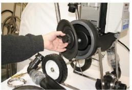
Rule 2. Before installing the new diaphragm, move the piston so it is fully withdrawn back into the pump frame. Removing the fan cover and rotating the fan by hand is the best way.
