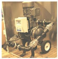
Step 1. Loosen both pump base v-clamps ( do not remove ) and rotate the suction, discharge and base assembly until the suction port is clear of the front support legs. Tighten the v-clamps.
