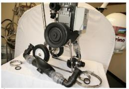
Step 3. Remove the Pump Base and Valves Assemby. Lay out all these parts for reassembly.
